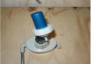
7. CAREFULLY Remove the pump skirt - Hold the plunger while unscrewing the large nut that encircles the plunger (it is spring-loaded! and will come out forcefully!). Remove the plunger, and place it on a clean surface (keep plunger clean).
