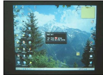
The power indicator light will start blinking. **DO NOT** remove the power cord from the projector or from the wall until the light stops blinking. This is very important!
