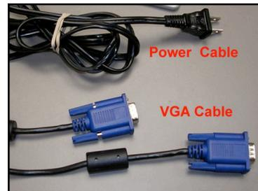
The VGA cable and power cord both connect to their corresponding ports on the back of the Video Projector.
