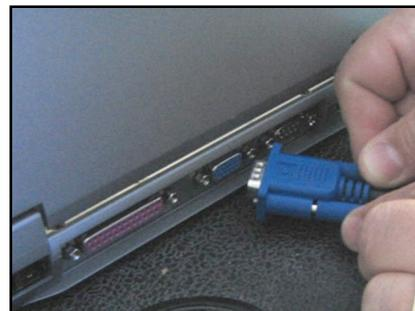
Make sure the monitor icon on the Apple VGA Display Adapter is facing up and gently insert the adapter into the port
