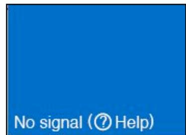
If you see a blank or blue screen or the “No Signal” message when you are connected to your Macintosh computer, press the Source Button on the top of the projector until it displays a message indicating Computer or Computer 1.
