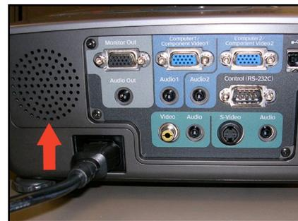
You will need an audio cable with a mini-plug at one end and 2 color-coded red and white RCA audio plugs at the other. (Note: Your model of projector or external speakers may use an audio mini-plug at both ends.)
