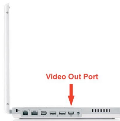
Make sure the monitor icon on the Apple VGA Display Adapter is facing up and gently insert the adapter into the port
