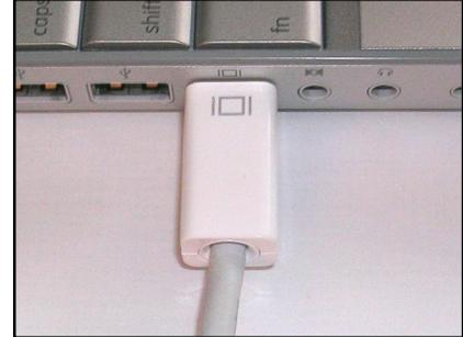
The Macintosh iBook's video-out port is "hot swappable" - which means you can take the Apple VGA Display Adapter out of the computer while the projector is on and connect it to another computer without having to change the settings on the projector itself. The projector will detect the new computer image automatically and project it.
