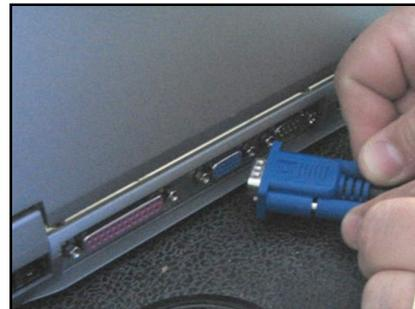
The video or monitor port on the Dell is also trapezoid shaped with 15 holes to accept the 15 pins of the VGA cable. It is also color-coded blue to match the VGA cable.
